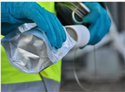
Slide the cartridges on the iFLUX Rod333, starting with the upper one. It's still important to not touch them.
