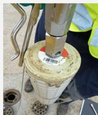
When the first 3 segments ( $\pm 1\text{m}$ ) are retrieved, block the string of samplers with the locking pin before unbolting the rods above.
