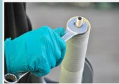
Secure the cartridges by tightening the nut at the lower end of the rod.
